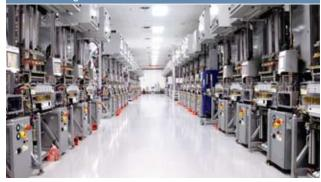
String Ribbon<sup>™</sup> wafers being "grown" in a patented quad furnace
