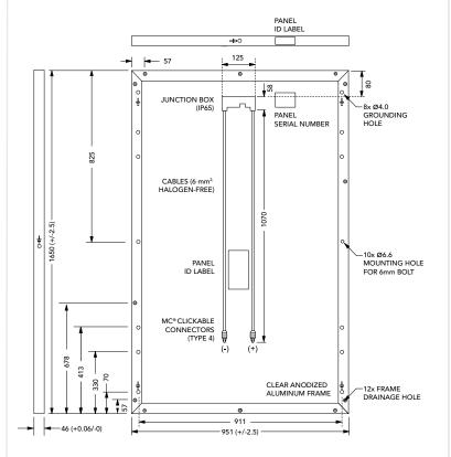
All dimensions in millimeters; panel weight 18.6 kg
