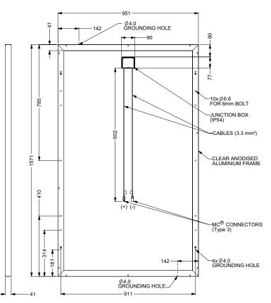
All dimensions in mm; module weight 18.2 kg
